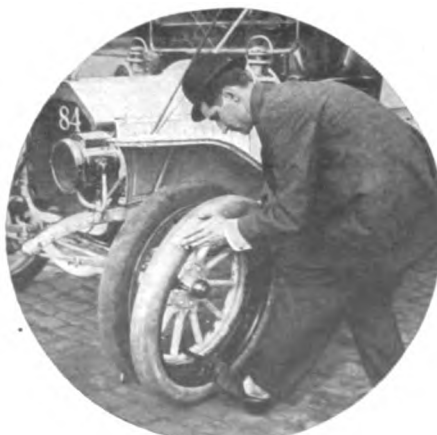
Fig. 2—Second operation, fitting emergency wheel in place
